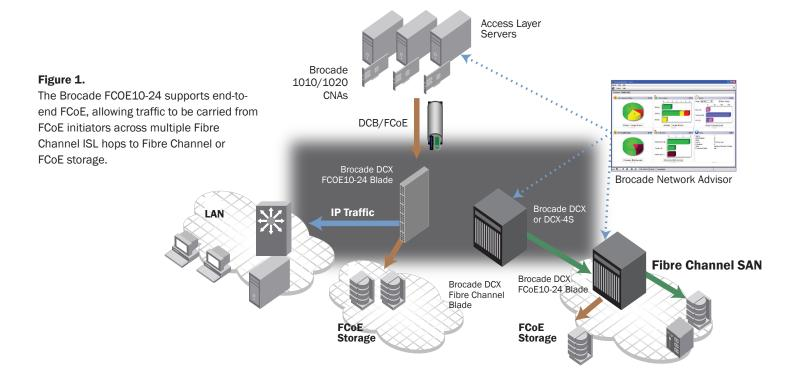
Its non-blocking architecture features 24 10 GbE DCB ports. Each Brocade DCX and Brocade DCX-4S chassis supports a maximum of four Brocade FC0E10-24 Blades, providing up to 96 10 GbE FC0E/DCB-capable ports per chassis.
