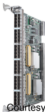
Figure 2. 8 Gbit/sec blades for the Brocade 48000 Director are available in 16-, 32-, and 48-port configurations.
