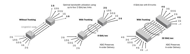
The Brocade 4100 utilizes new ASIC technology featuring four 8-port groups. As a result, an Inter-Switch Link (ISL) trunk can have up to eight ports supplying as much as 32 Gbit/sec of data throughput (see Figure 1). In addition to reducing congestion between switches and providing greater total bandwidth, enhanced ISL Trunking utilizes ISLs more efficiently to free up the number of usable switch ports.
